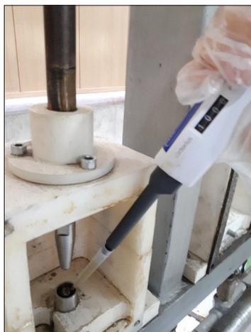
**Figure 1:** Microbial solution recharge during cyclic load
